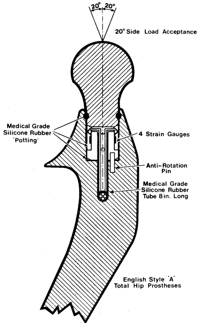
Fig. 7. Cross-sectional view of prosthesis head/neck
