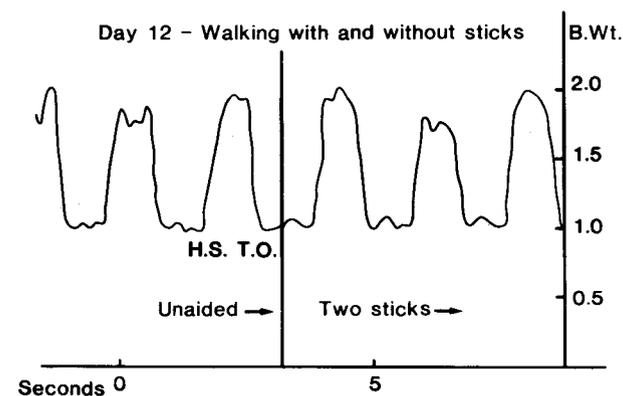
Fig. 15b. Load recording during walking with and without sticks
