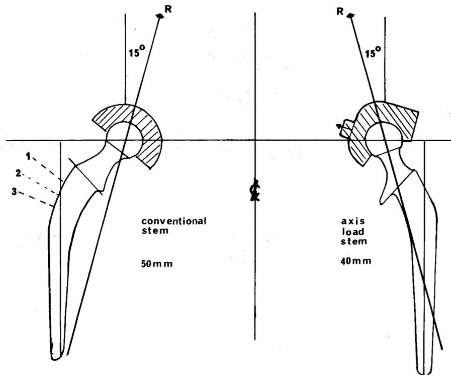
Fig. 1. Resultant load directions axial and conventional prosthesis
