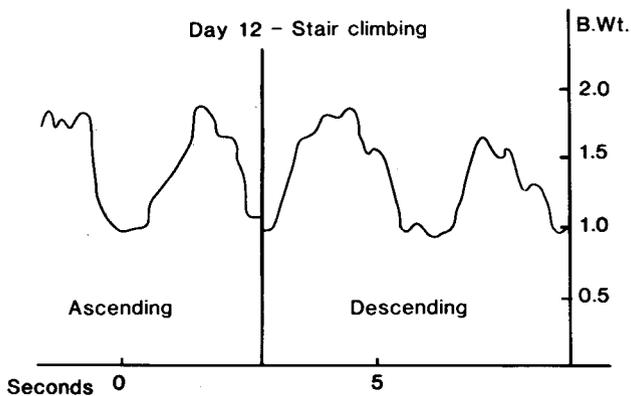
Fig. 15a. Load recording during stair climbing
