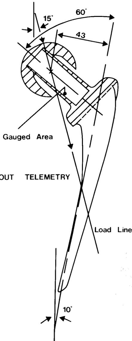
Fig. 2. Rydell strain gauged prosthesis (1966)
