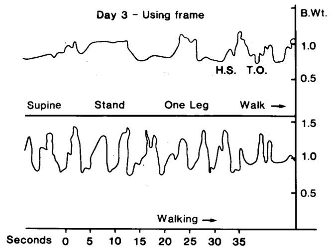
Fig. 14d. Load recording during first assisted walking attempts
