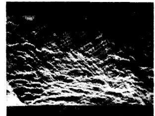
Fig. 3c. Fatigue striations on fracture surface (B. A. Jordon, AWRE 1976)
