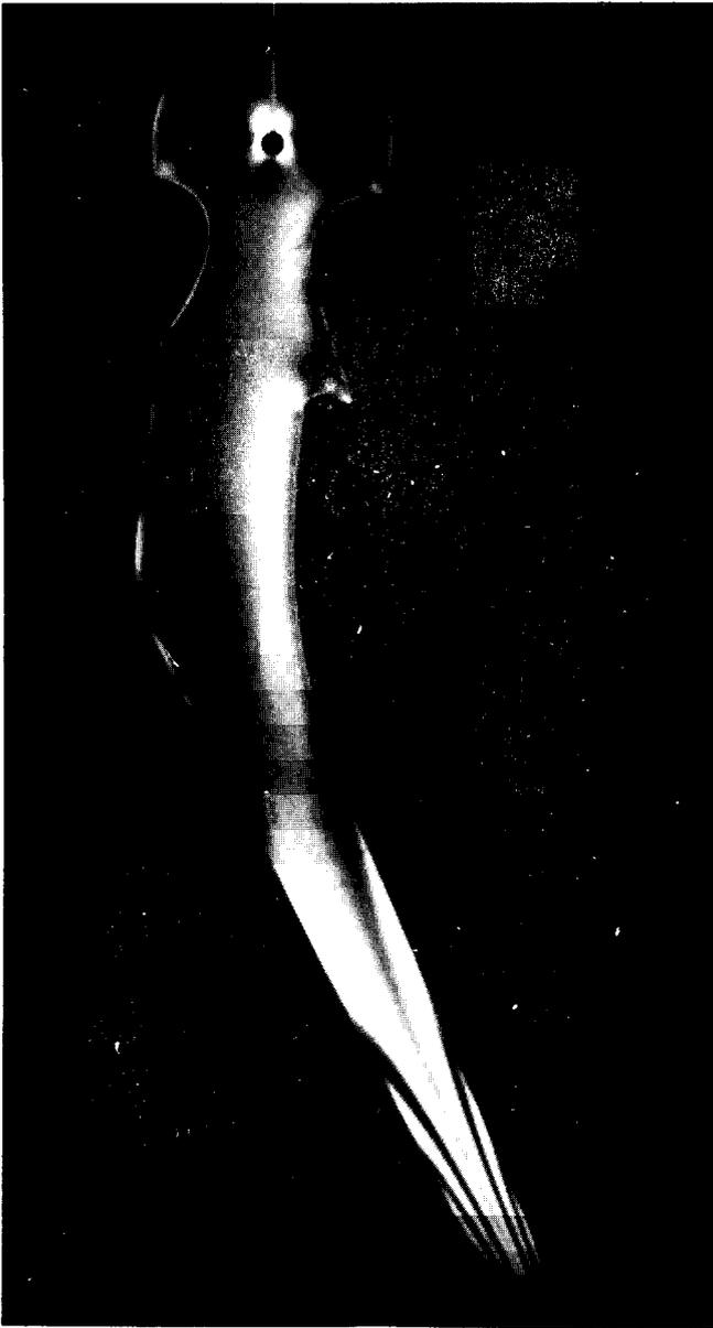
Fig. 6. Photo-elastic model of prosthesis under axial loading
