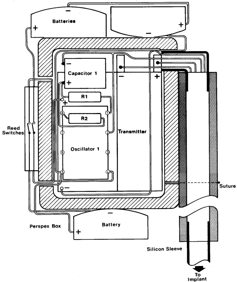
Fig. 9. Layout of implanted electronics package
