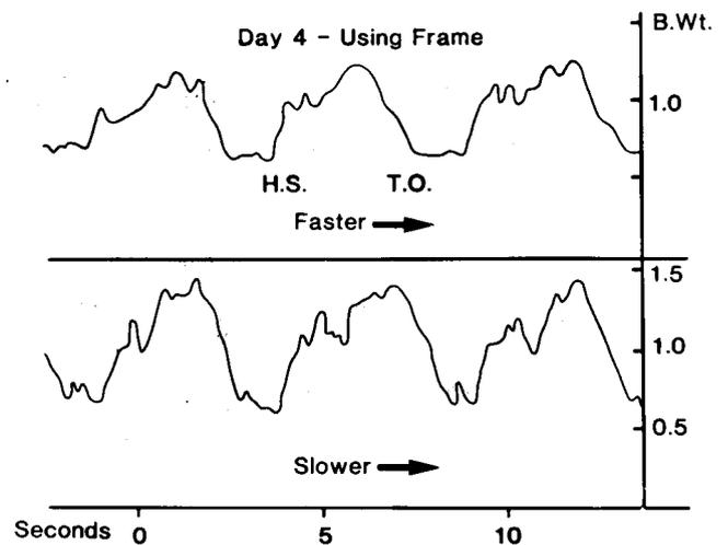
Fig. 14e. Load recording during assisted walking
