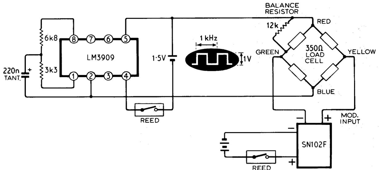
Fig. 8. Transmitter circuit diagram
