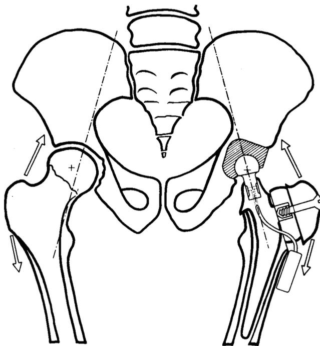
Fig. 5. Method of measuring the prosthesis axial force
