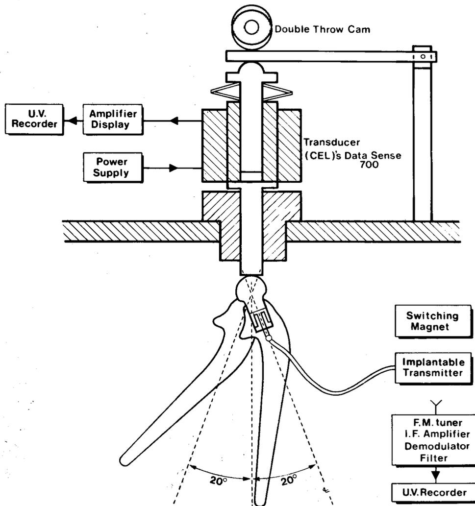
Fig. 12. Calibration method
