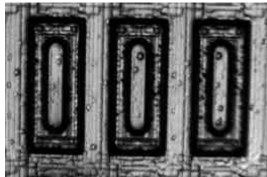
Figure 3 Picture of three sensor sites after the electroless gold plating. The central bars are the switched output node of each individual sensor. The surrounding conductor is a common ground. The sensor material is deposited on top of the chip, forming the sensor between the central contact and the surrounding ground
