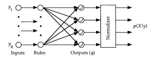
Figure 2.1: Rule-based classification network
