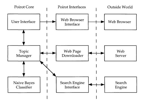
Figure 4.1: System block diagram for the autonomous agent called Poirot
